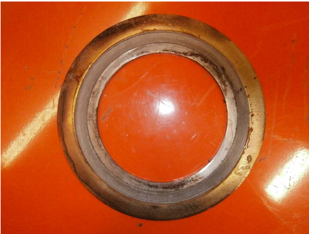
Test Gasket Post-Burn
