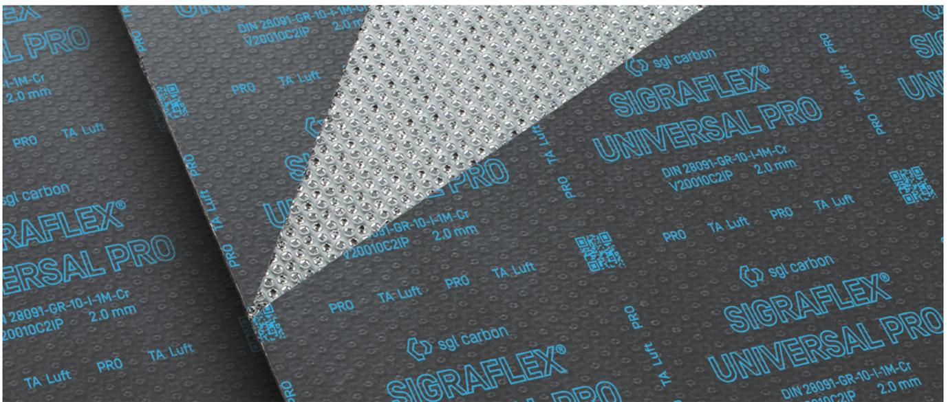
SIGRAFLEX UNIVERSAL PRO is an adhesive-free graphite sealing sheet made from flexible graphite foil with one or two tanged stainless steel reinforcements. The sealing sheet is impregnated to reduce leakage and improve handling.
