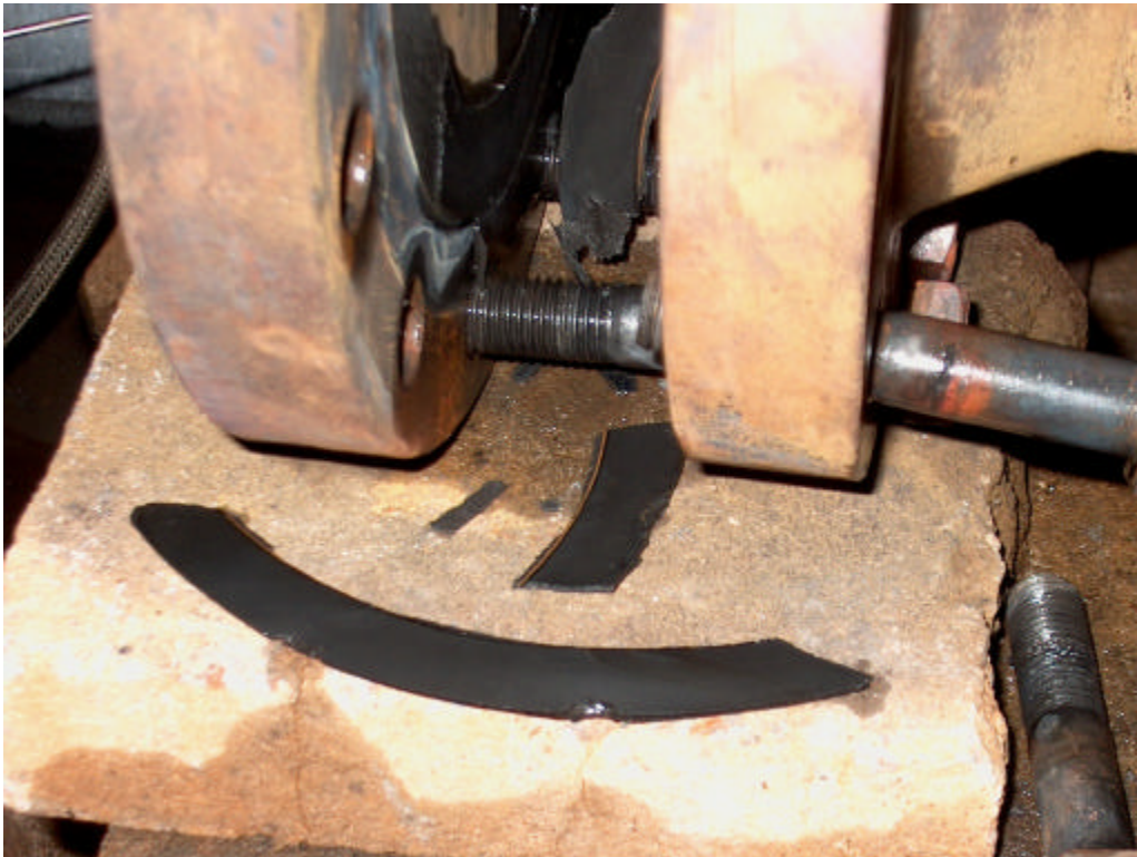
(Upstream Leakage) Gaskets After Test
