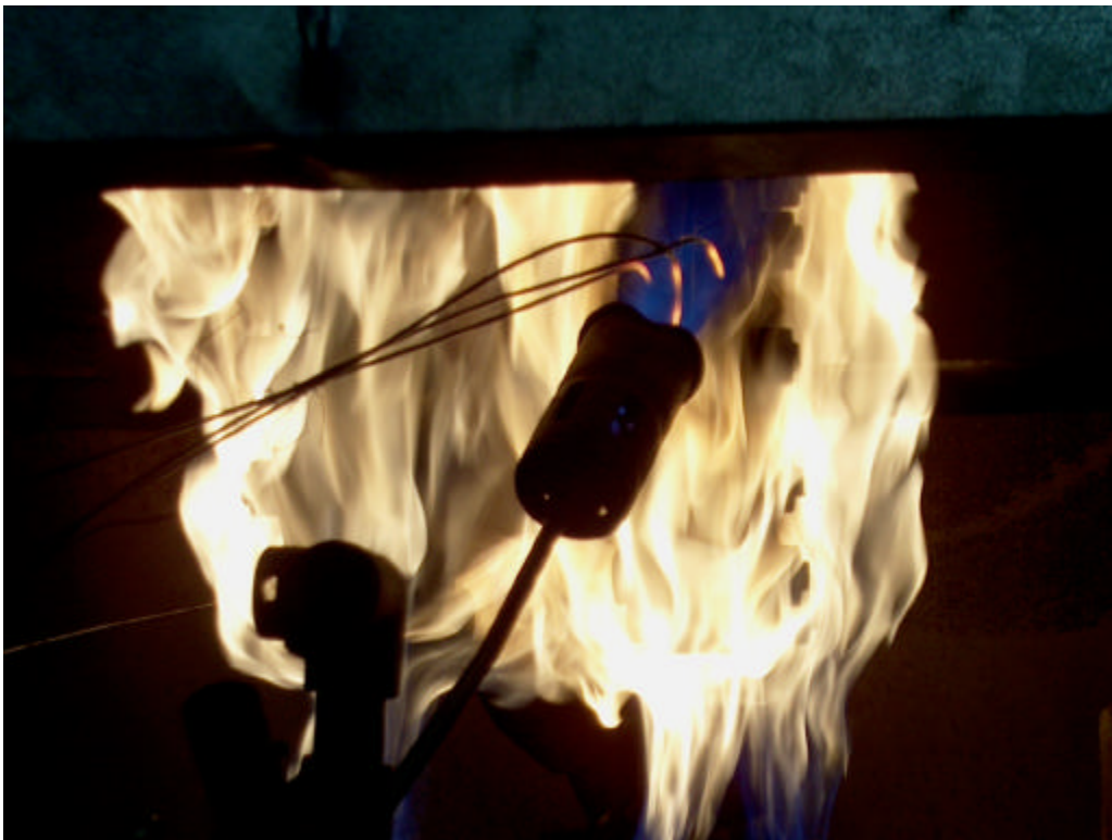
Flange Assembly During Burn
