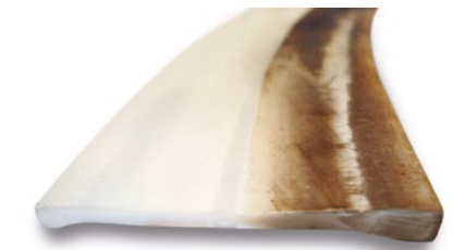
Cross section of GORE® Gasket Tape Series 1000 after service in challenging process conditions
